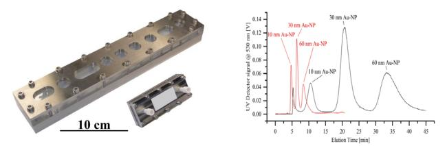
Figure 2: Photograph (left) shows the difference in dimensions of the mAF4 cartridge when compared with the conventional analytical AF4 cartridge. The graph (right) shows the respective particle size fractograms obtained using the two cartridges for a mixture of gold nanoparticles (10 nm, 30 nm, 60 nm). (With permission from [6]).
