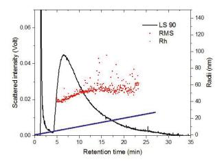
Figure 2: AF4-MALS fractogram of the CNC sample and R.M.S and Rh radii profiles
