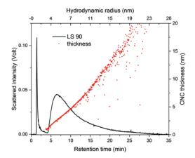
Figure 3: CNC length distributions obtained from AFM and AF4-MALS (left). CNC thickness profile as a function of retention time and hydrodynamic radius (right)
