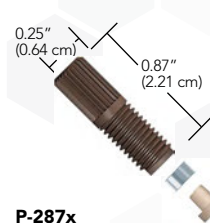
P-287x (1/4-28, ≤ 1/16" OD Tubing) P-387x (1/4-28, > 1/16" OD Tubing)
