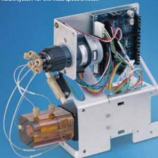
A configuration of the Controlled Delivery Module enabled development of the fluidic system for the mass spectrometer.
