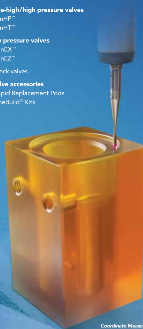
Coordinate Measurement Machine inspection of pump housing
