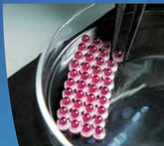
100% leak testing of ruby ball/valve seat assemblies prior to packaging
