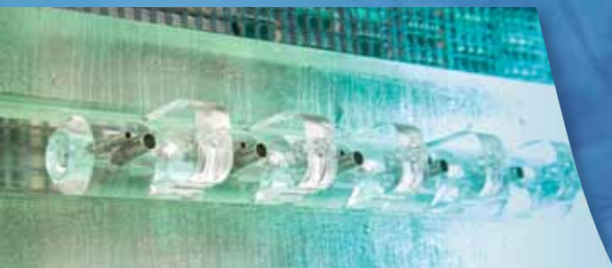
Ultraviolet curing of bonded tubing inserts
