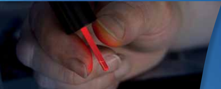
100% visual inspection of IDEX Health & Science ultrahard HPLC components rejected this flawed ruby piston
