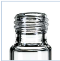
Short Thread ND9 (Thread ends in the middle of the neck, so that there is still some space between the edge of the cap and shoulder of the vial for robotic arms)
